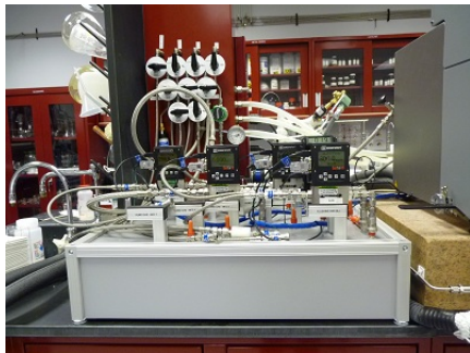
Gas Delivery System
